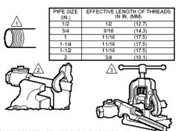
USE PROPERLY REAMED AND CLEANED PIPE AND MODERATE AMOUNT OF DOPE (LEAVE TWO THREADS BARE)
