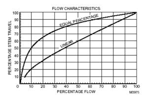
Fig. 2. Equal percentage and linear flow characteristics.
