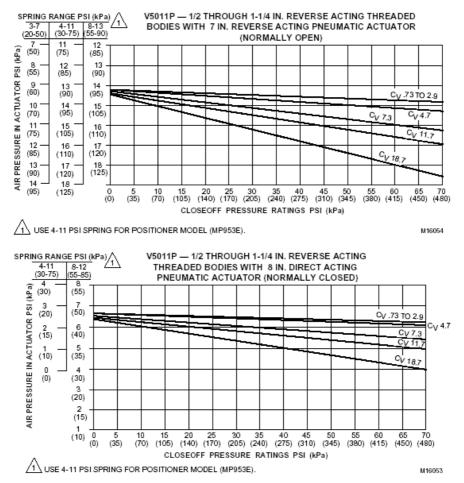
Fig. 3. Close-off ratings at various control air pressures for V5011P Valves and MP953 Pneumatic Actuators. (continued)
